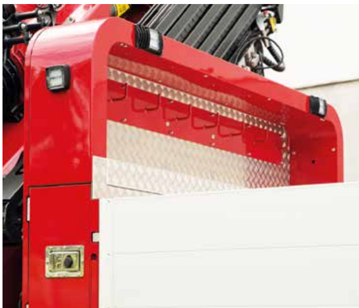
FUNCTION AND DESIGN OF BULKHEAD
